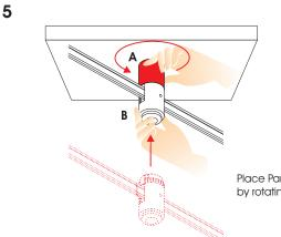
Place Part B back on and tighten it carefully by rotating clockwise only part A.
